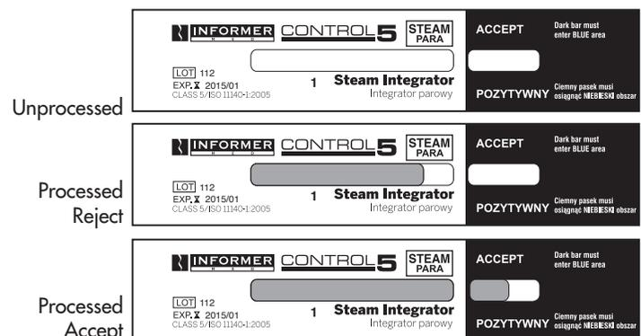
If the dark bar has not reached the *accept* window adequate sterilization conditions are not satisfied. Material should be reprocessed.
